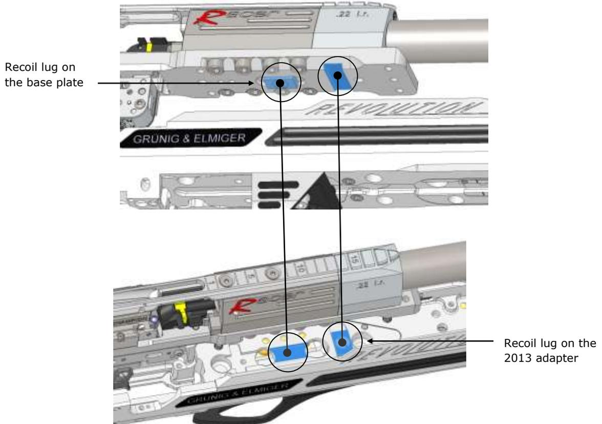
Carefully join the system and aluminum stock!
