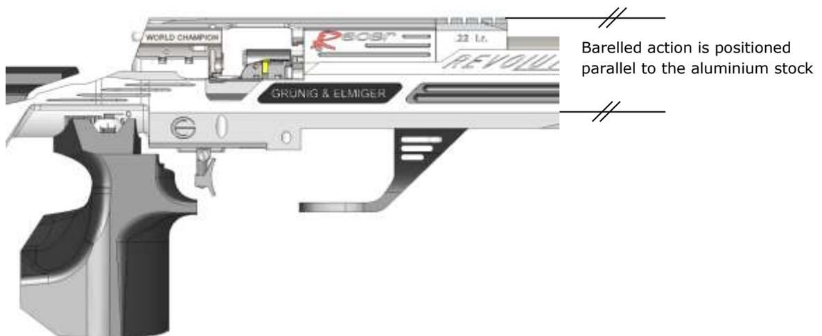
Squeeze the barreled action and the aluminum stock together with your hand (as illustrated below) and then hold it upright. You can now insert the action screws and turn them only as far as you feel little resistance. Do not yet tighten the action screws. By its own weight, the base plate will align itself correctly with the 2012-adaptor. Continue to hold the aluminum stock upright.
