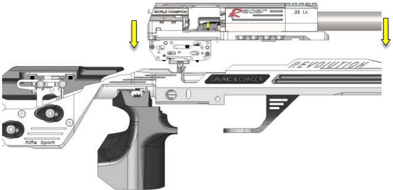
The barreled action is now positioned correctly in the aluminum stock. Check if the barreled action is parallel to the aluminum stock (see picture below).
