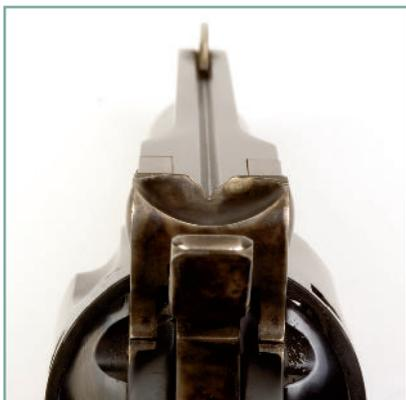
*The rear sight is a V-shaped notch cut into the barrel latch. Note the groove that runs along the top of the barrel. Both the rear sight and the front sight are fixed, so any adjustments will have to be made with a file.*
