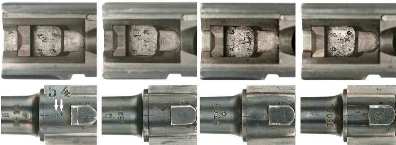
Fig. 9-96: From early 1914 the letter N became the principal inspection mark on all production, being generally applied in the frame well and on the receiver stop lug. Top left , undated long-frame Naval P.04 without grip-safety, sn. 5432b, retaining two additional serial number digits on the receiver ring; top right , 1916 dated P.04 on which, despite the attempts to rationalise production, the last two digits of the serial number were still stamped on the stop-lug in the commercial style, although the additional digits on the receiver ring of 1910 - 14 production are now omitted; bottom left , P.08 sn.5709o/1916, marked N in both locations and with no internal serial numbering, as with all P.08s from 1911; bottom right , commercial P.08 sn. 76062 marks the end of WWI commercial production in 1916 and also the use of the N mark, with similar inspection marks and retaining commercial pattern two digit receiver serial numbering on the stop lug as the 1916 dated P.04s.
