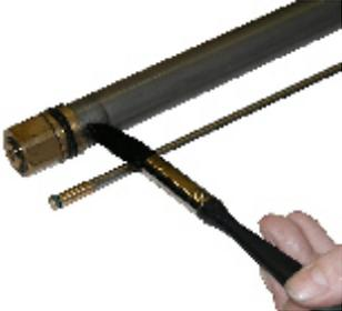
Having cleaned the components and replaced the seals apply a small amount of silicone grease to tube, piston rod, large o'ring and green o'ring on piston.
