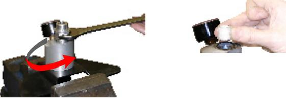
Hold the footplate in the vice and using a suitable spanner unscrew the non return valve from manifold block (anticlockwise) and place to one side. Lift out the filter element from the body of the manifold block and replace with new one. Use long nose pliers if difficult avoiding damage to threads
