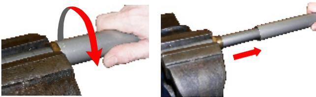
Using the vice, gently clamp the brass gland nut (not the inner tube) at bottom of the painted outer tube. Gripping the tube, unscrew anticlockwise. The painted tube can now be removed from the pump.
