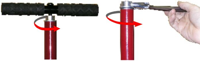
Grip the pump body and spin off the handle (anticlockwise). Using the spanner flats and suitable size spanner, unscrew the handle connector.
