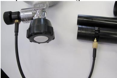
Close the valve of the pressure bottle (pressure cylinder), and release the excess air by the safety valve (the smaller circle).
