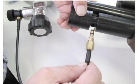
Check the closure of the safety valve of the pressure (the smaller circle) and open the valve of the pressure bottle (pressure cylinder) (the bigger circle).
