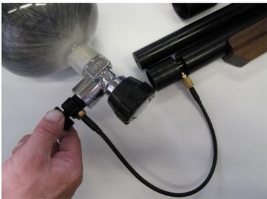
Remove the the tube from the pressure container on the gun.
