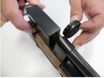
Set the MLC into one of the two positions and by the rotating of the magazine find the position when is fixed.
