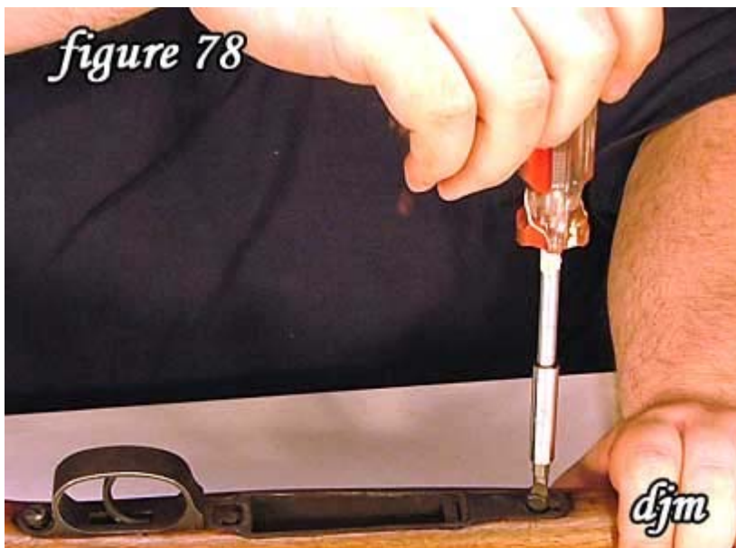
78) Tighten partially the forward guard screw.
