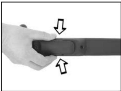
Press the two snap latches at the right and the left of the magazine fully together using thumb and index finger of one hand and remove the magazine while pressing.
