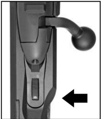
The safety can be operated only when the weapon is cocked or the bolt handle is open!
