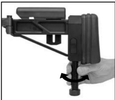
Additional the shaft can be extended at 30mm / 1,2" by turning out the spike.
