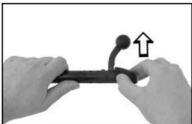
Grip the bolt with your left hand. Push in catch lever with your right thumb and simultaneously rotate the bolt sleeve clockwise (arrow shows direction of rotation) until it unlocks with an audible click. Take off bolt sleeve and extract firing pin assembly.
