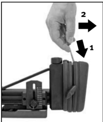
The butt plate can be removed using a screw driver. The length of pull may be adjusted individually by means of spacers.
