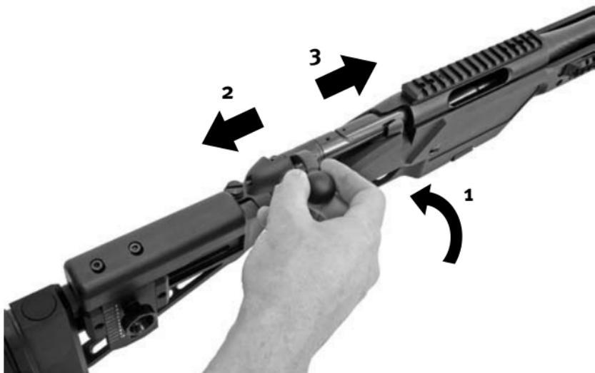
Turn bolt handle  $70^\circ$  upwards to unlock the bolt. Pull bolt all the way to the back by the bolt handle. When moving the bolt forward, a cartridge will be fed into the cartridge chamber of the barrel and by turning the bolt handle down, the action will be locked.
