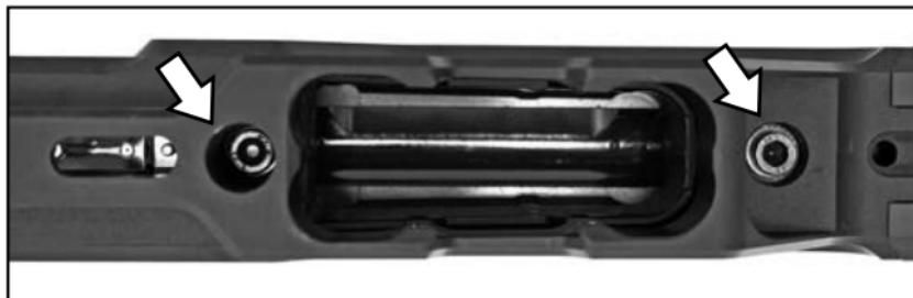
If these screws are loosened, they have to be retightened again with a torque wrench ( $7 \text{ Nm}$ ).
