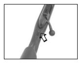
Turn bolt handle 70° upwards to unlock the bolt. Pull bolt all the way to the back by the bolt handle.
