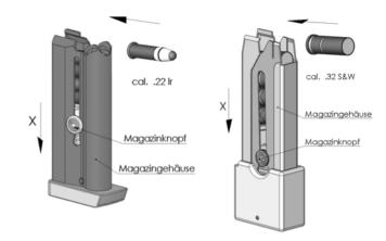
When sliding the cartridges into the magazine (direction of arrow) ensure that you slide them in the right direction and that the cartridges in the magazine do not snag (bottom rim of the cartridge). It is easier to slide the cartridges in if slight pressure is exerted at the same time on the button of the magazine (arrow direction X).
