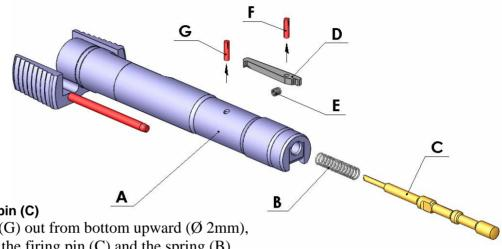
Removing the firing pin (C)
