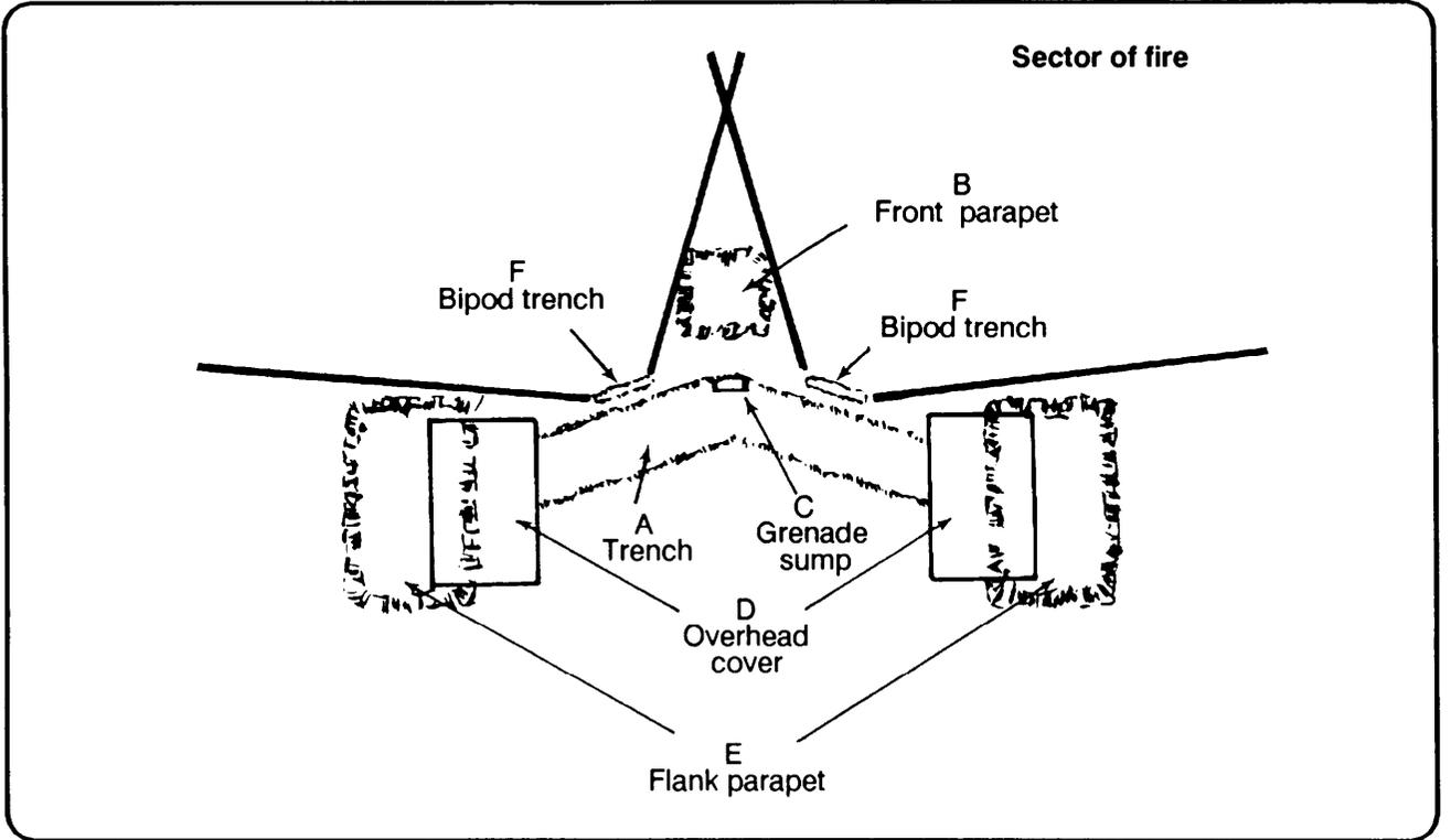
Figure 3-10. Construction of a two-man fighting position.
