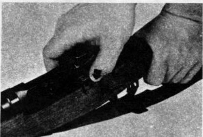
Figure 5. Locking the bolt to the rear.
