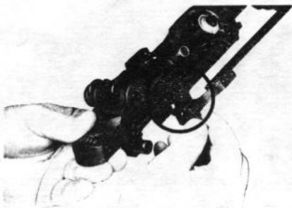
Figure 13. Removing operating rod.
