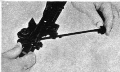
1 Figure 17. Replacing the connector assembly.
