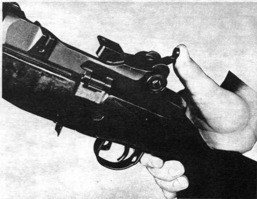
Figure 47. Adjusting sight tension.
