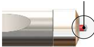
Firing pin cocked but secured
